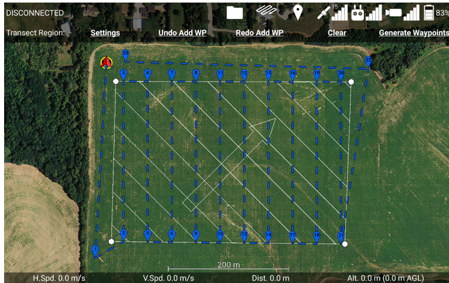
Figure 97: You can change the orientation and spacing of the transect lines even after generating waypoints.
