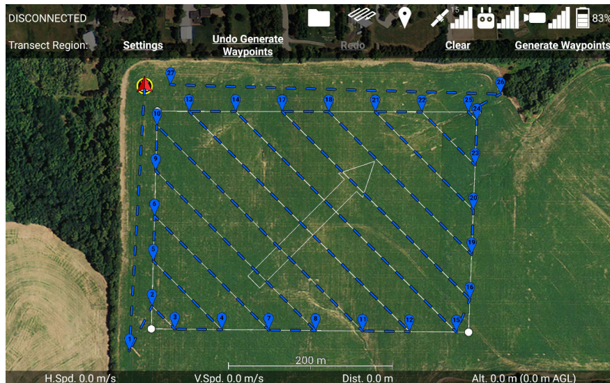
Figure 98: Newly generated waypoints will replace the part of your waypoint mission that passes through the transect region.
