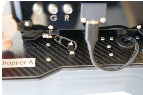
Figure 28: Attaching the front tether to the front connection point on the dropper. Clip the back tether to the back connection point.
