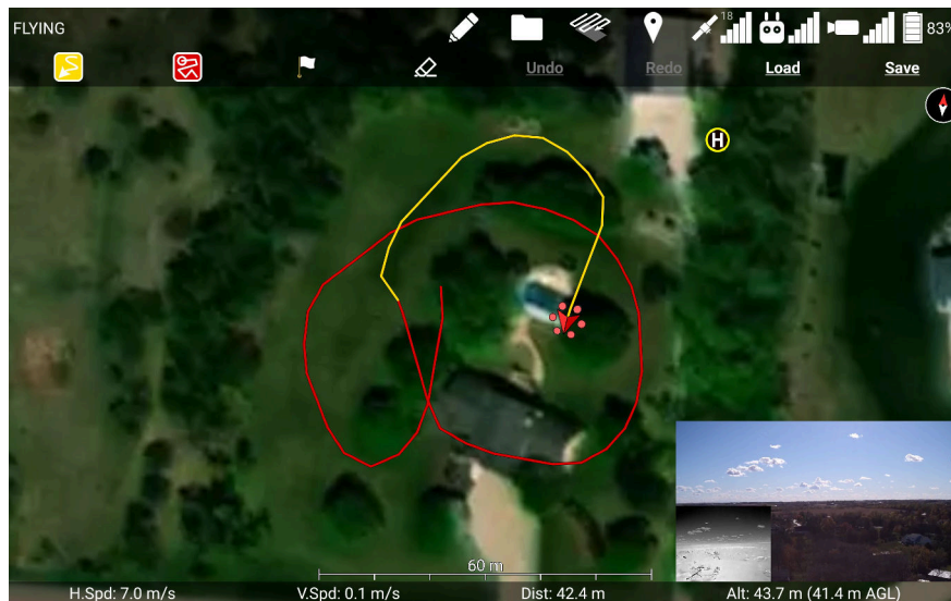
Figure 108: Using the drone to draw a line on the map. The color was changed from red to yellow mid-way through.
