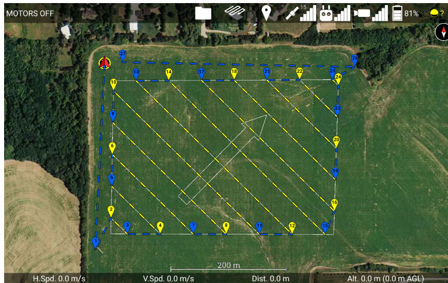
Figure 99: When the usage is set to Ignition, the generated waypoints will be automatically activated for dropping along the transects.
