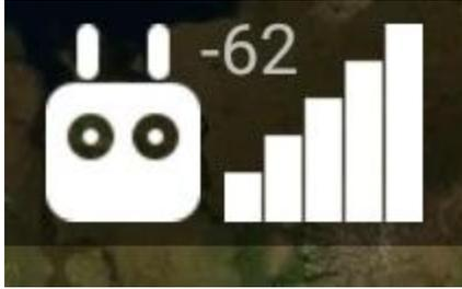
The bars next to the controller in the app show the percentage of the flight controller's Mavlink packets that are making it to the app. This is helpful for detecting end-to-end communication problems, including ones caused by software problems, but it doesn't really drop off with range until you're at the limit.
