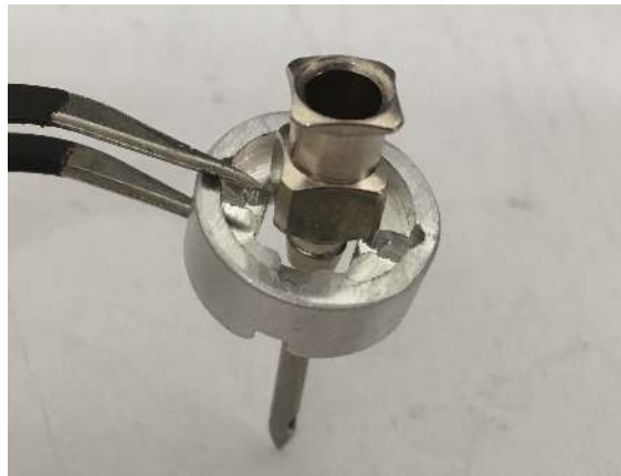
Figure 94: Slide the retainer over the new needle.
