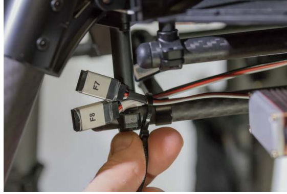
Figure 104: Ziptie the connectors in place.
