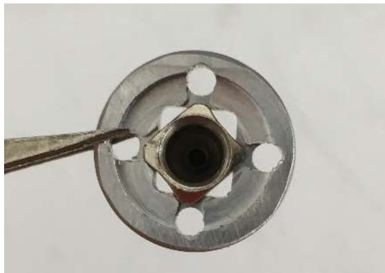
Figure 96: Needle tabs aligned with the cutouts on the retainer.
