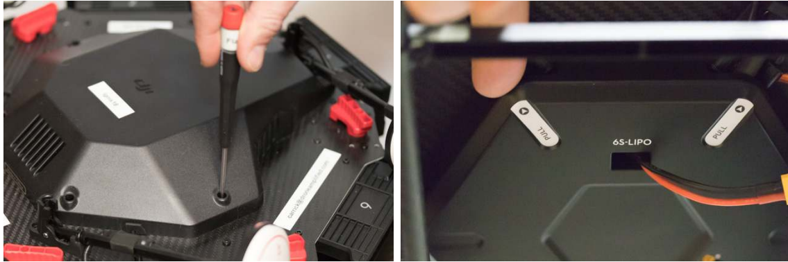
Figure 100: Unscrew top cover and remove bottom cover.
