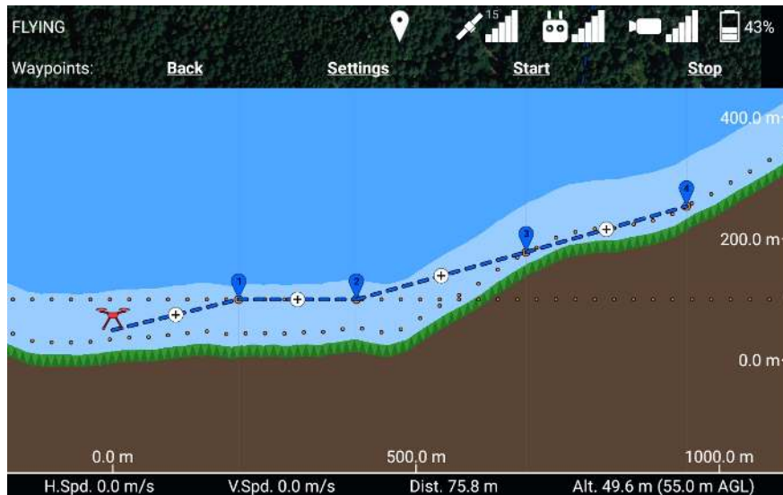
Figure 84: Snap altitudes are shown as dotted orange lines. Newly placed waypoints will be placed at the higher of the snap altitudes, and when you adjust the altitude of a waypoint, it will “snap” to the snap altitude lines if it is moved close to one of them.
