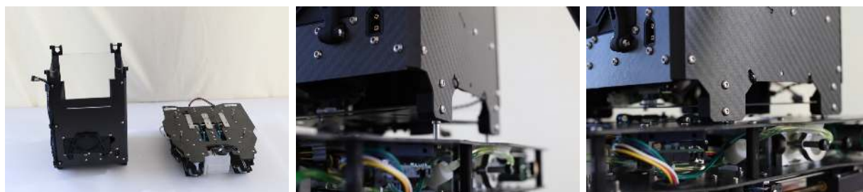
Figure 8: Attaching the Dropper to the Hopper.
