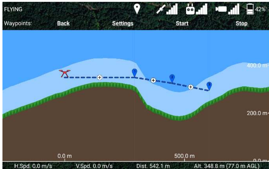
Figure 80: Touch the plus button in the middle of a waypoint path segment to create a new waypoint there.
