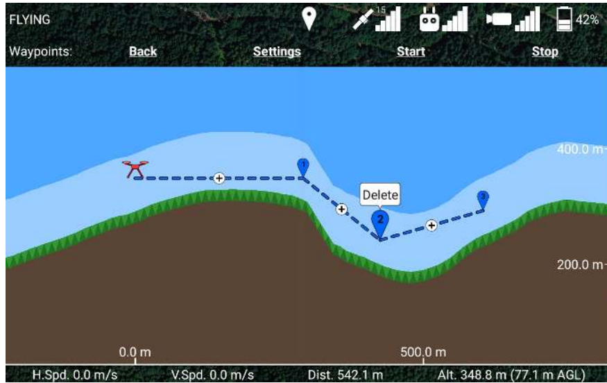
Figure 84: If you briefly touch a waypoint, it will give you the option to delete it. Touch the “Delete” bubble above the waypoint to confirm the deletion of it, or touch anywhere else to deselect it.
