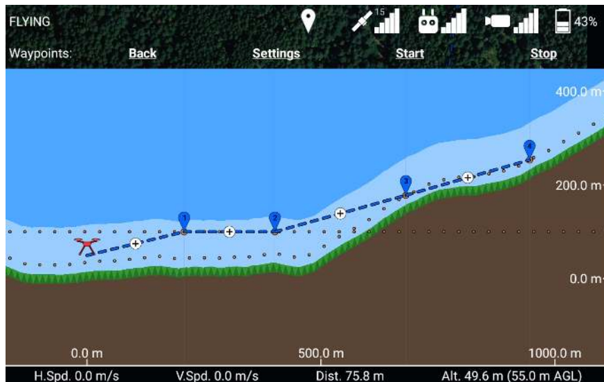
Figure 86: Snap altitudes are shown as dotted orange lines. Newly placed waypoints will be placed at the higher of the snap altitudes, and when you adjust the altitude of a waypoint, it will “snap” to the snap altitude lines if it is moved close to one of them.
