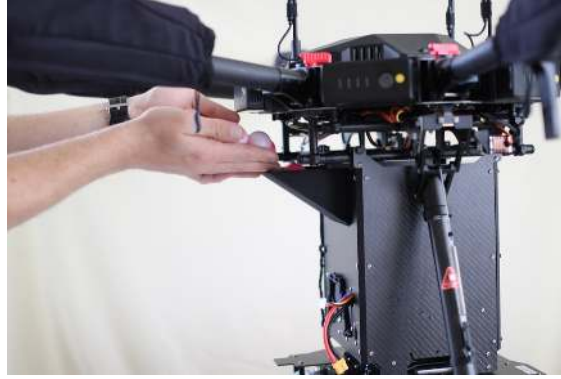
Figure 30: Filling the Hopper with ignition spheres.
