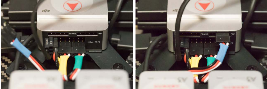
Figure 104: Three connectors installed.
