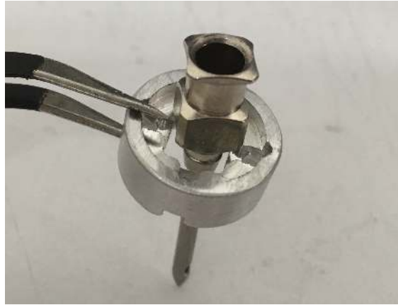
Figure 96: Slide the retainer over the new needle.
