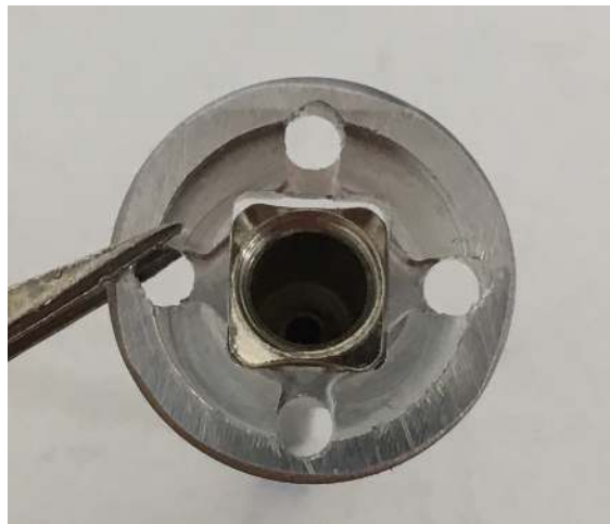
Figure 97: The needle can only fit through the rectangular hole in one orientation.
