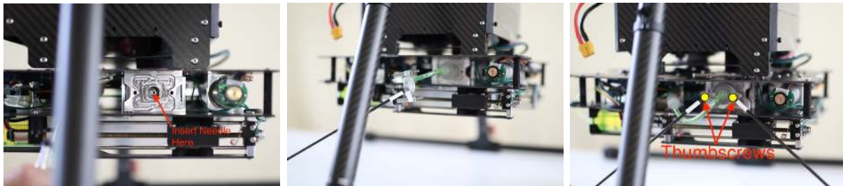
Figure 112: Left: Location to insert the needle. Center: Needle assembly holder. Right: Needle assembly holder in place.
