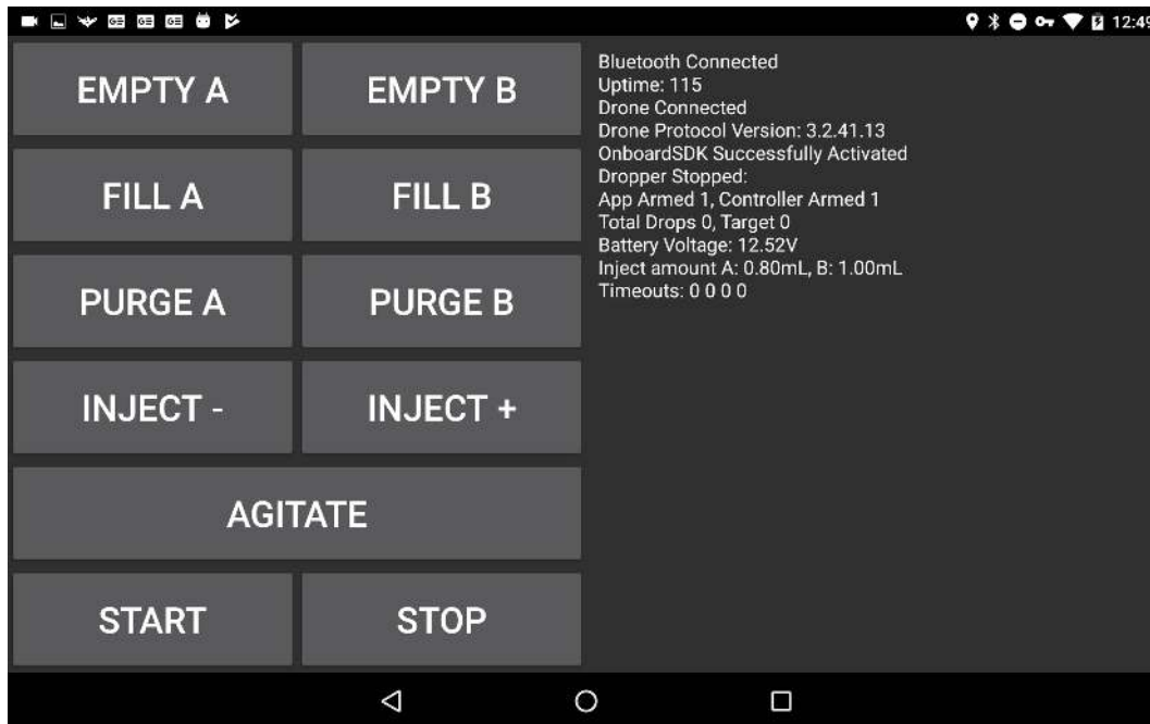
Figure 110: Message displayed when the DJI Onboard SDK is Successfully Activated
