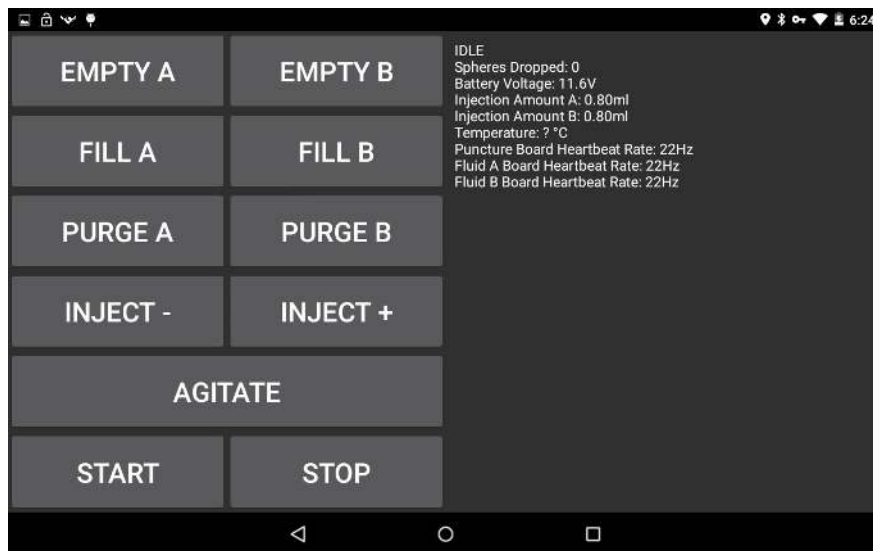
Figure 58: App when connected to Ignis through the Drone.
