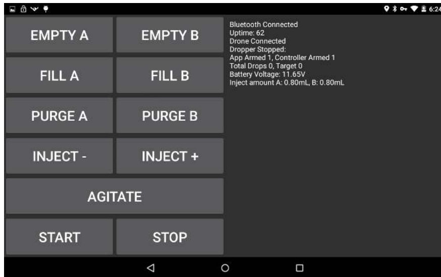
Figure 17: App when connected to Ignis.
