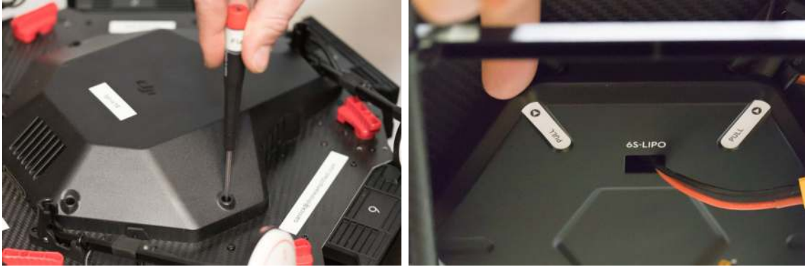
Figure 122: Unscrew top cover and remove bottom cover.
