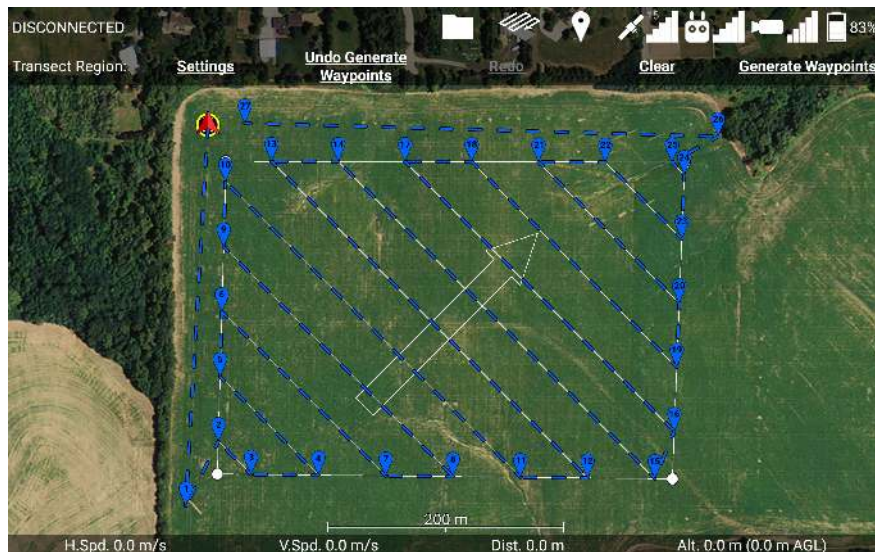
Figure 102: Newly generated waypoints will replace the part of your waypoint mission that passes through the transect region.
