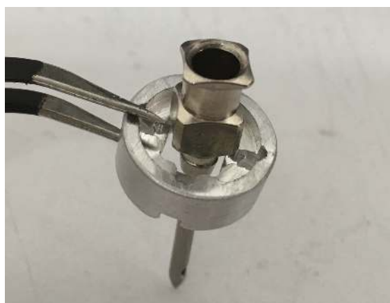
Figure 116: Slide the retainer over the new needle.
