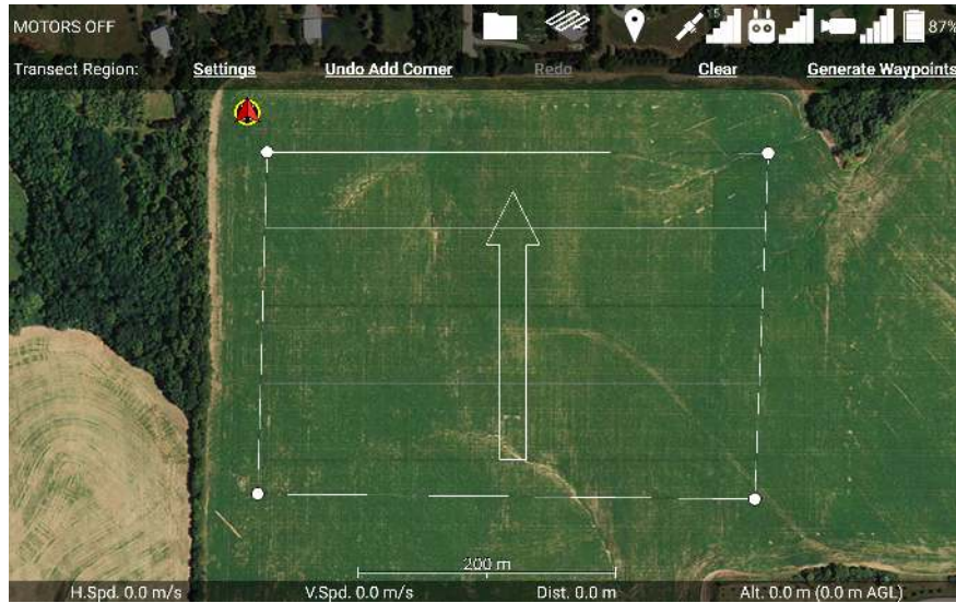
Figure 96: Touching the map while in the transects menu will define the corners of the transect region.
