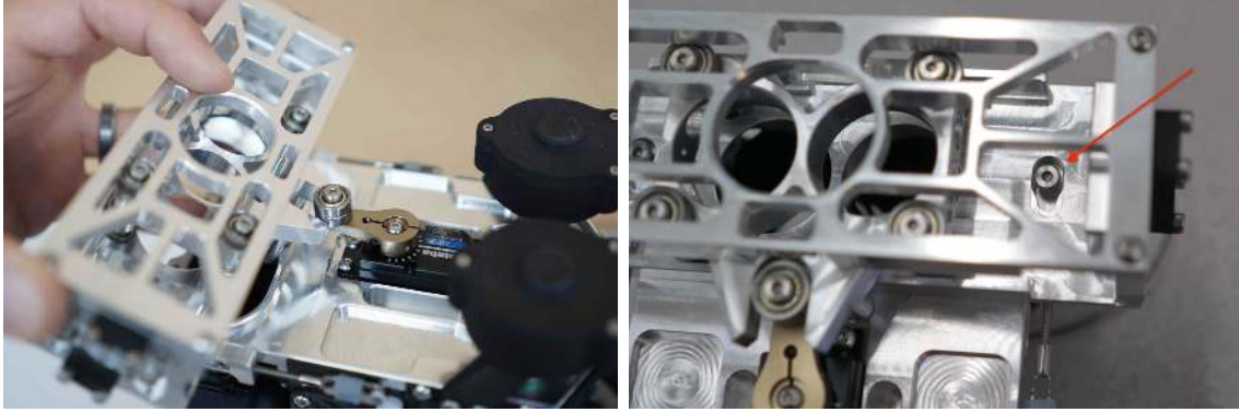
Figure 12: Attaching the Dropper to the Hopper.
