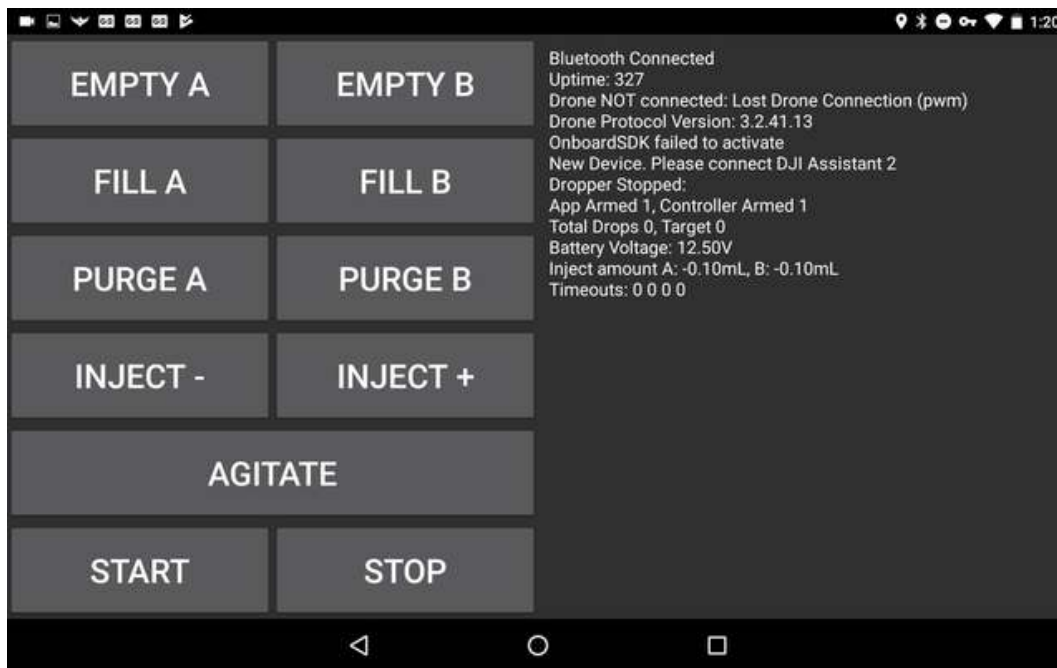
Figure 129: Error message displayed when the Matrice 600 has not performed the DJI Onboard SDK Activation with Ignis
