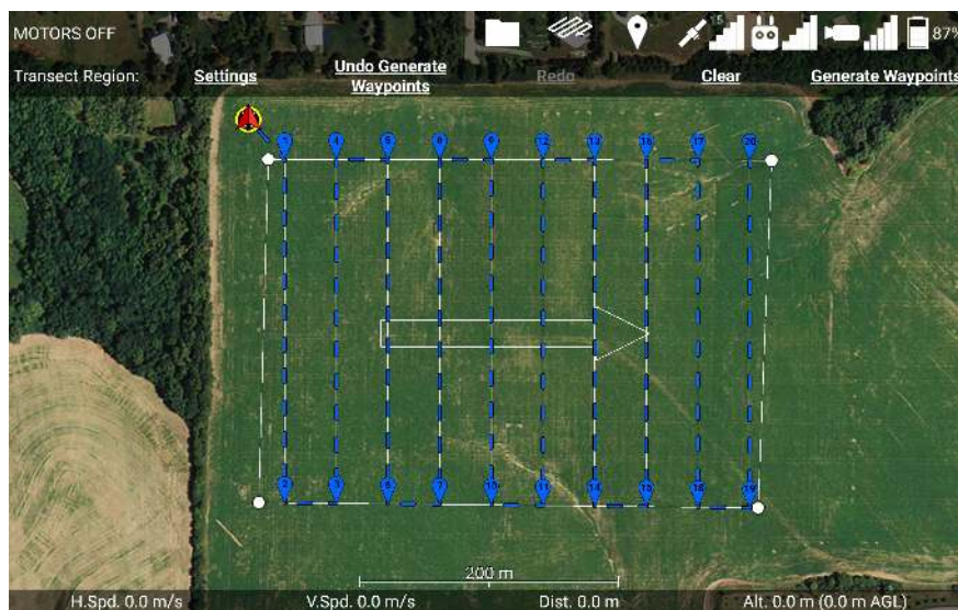
Figure 98: Touch the Generate Waypoints button to generate waypoints that follow the transects.
