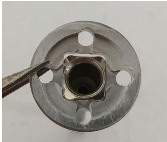
Figure 117: The needle can only fit through the rectangular hole in one orientation.
