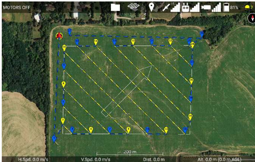
Figure 103: When the usage is set to Ignition, the generated waypoints will be automatically activated for dropping along the transects.
