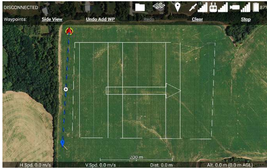
Figure 99: Place waypoints to define a custom ingress route to the transect region.
