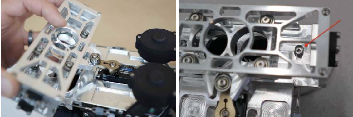
Figure 12: Attaching the Dropper to the Hopper.
