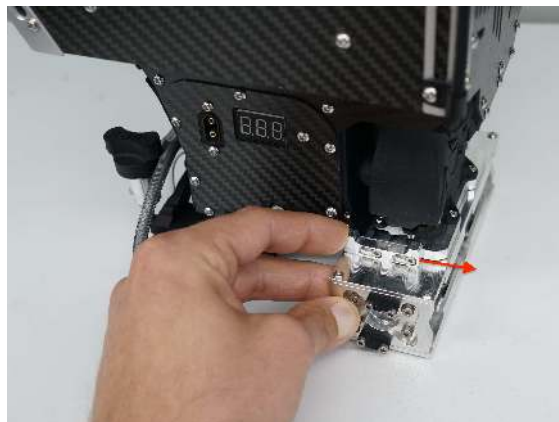
Figure 40: Manually separate the Dropper by sliding the emergency release bracket on both sides of the dropper forward
