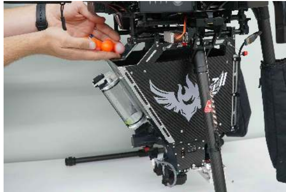
Figure 38: Filling the Hopper with ignition spheres.
