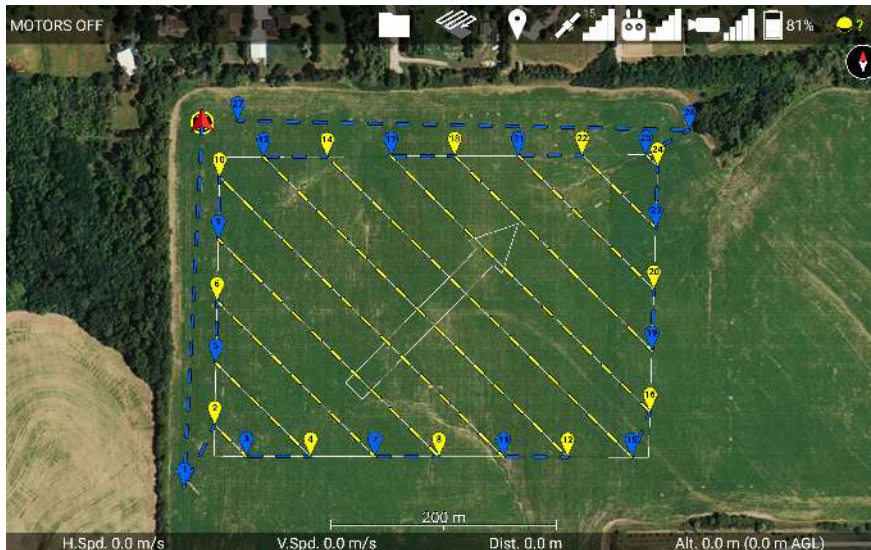
Figure 105: When the usage is set to Ignition, the generated waypoints will be automatically activated for dropping along the transects.
