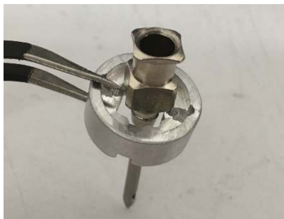
Figure 118: Slide the retainer over the new needle.
