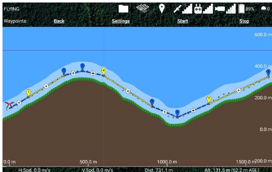
Figure 96: You can also toggle dropping along lines by touching them in the side view.
