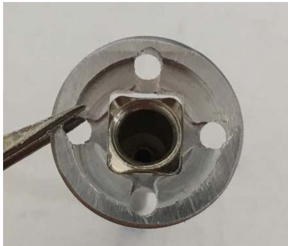
Figure 119: The needle can only fit through the rectangular hole in one orientation.
