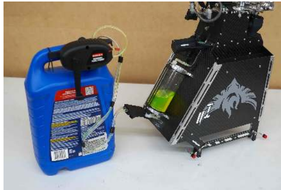
Figure 42: Turn Ignis upside down and connect the fill coupler to prepare to empty the reservoir, pumps and tubing
