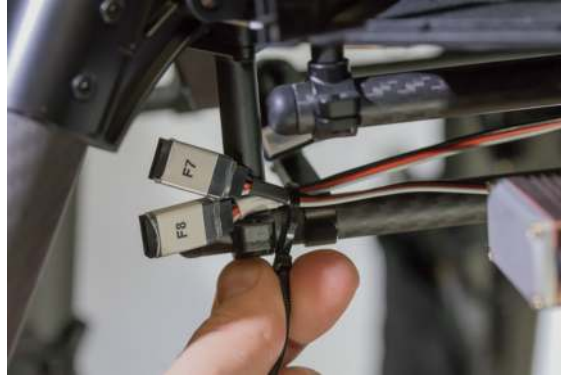
Figure 128: Ziptie the connectors in place.
