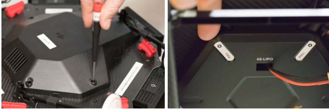
Figure 124: Unscrew top cover and remove bottom cover.
