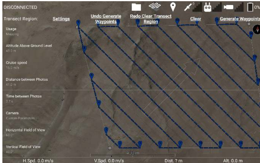
Figure 106: When the usage is set to Mapping, you'll see additional controls to help you design a mission that will yield overlapping photos.
