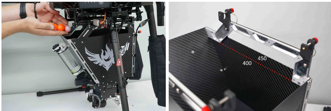
Figure 31: Left: Filling the Hopper with ignition spheres. Right: Approximate capacities.
