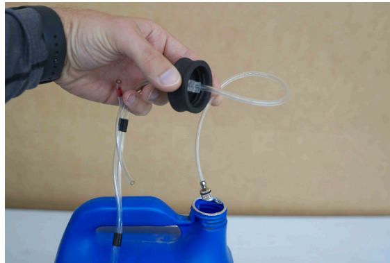
Figure 6: Put pickup clunk and tube into jug first and tighten cap.
