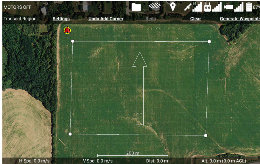
Figure 98: Touching the map while in the transects menu will define the corners of the transect region.
