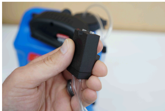
Figure 24: Proper grip on fill coupler
