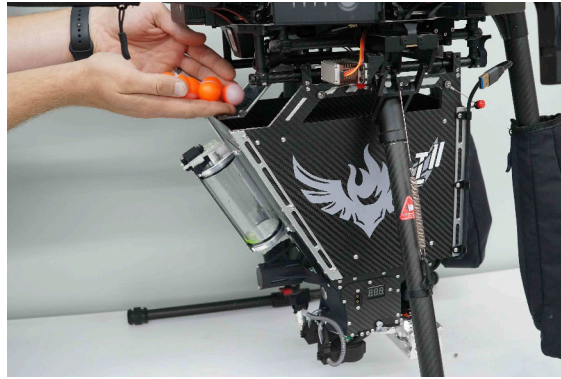
Figure 38: Filling the Hopper with ignition spheres.
