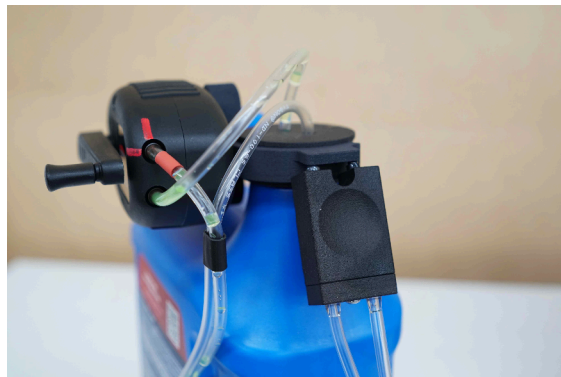
Figure 26: Store the coupler on the antifreeze jug between uses to prevent contamination from dirt and to prevent siphoning.
