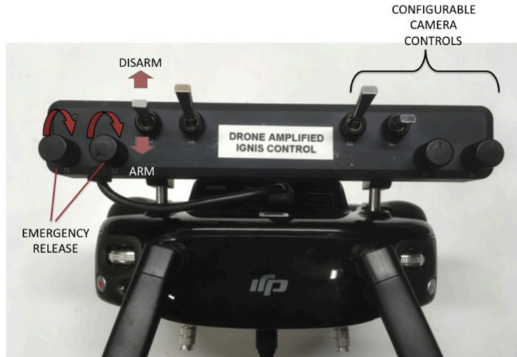
Figure 4: Ignis control switches.
