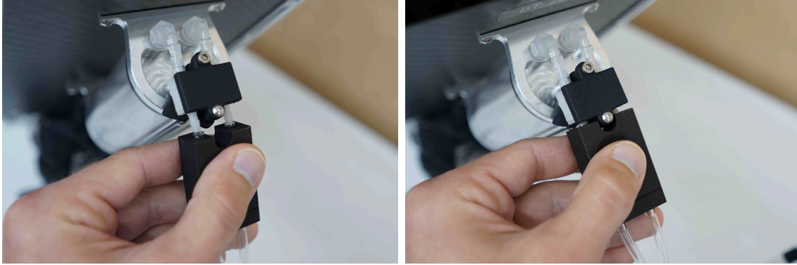
Figure 25: Left: Align the tubes on the coupler with the check valve barbs. Right: Press the coupler onto the reservoir until it stops.
