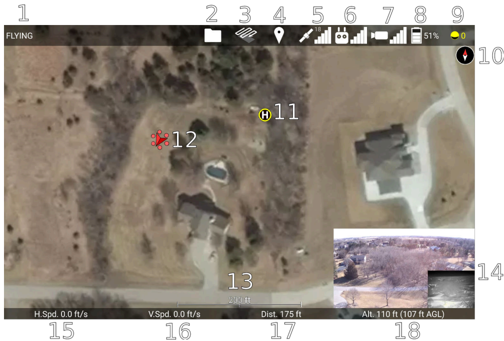
Figure 70: Main interface elements while flying.
