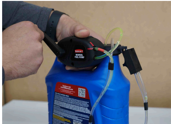
Figure 23: Prime pump by cranking rapidly clockwise until antifreeze enters pump
