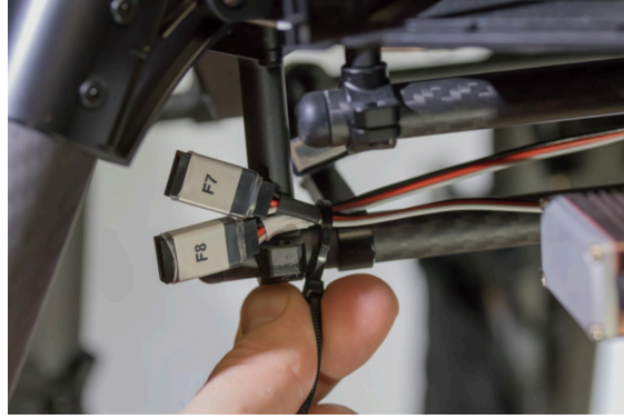
Figure 129: Ziptie the connectors in place.
