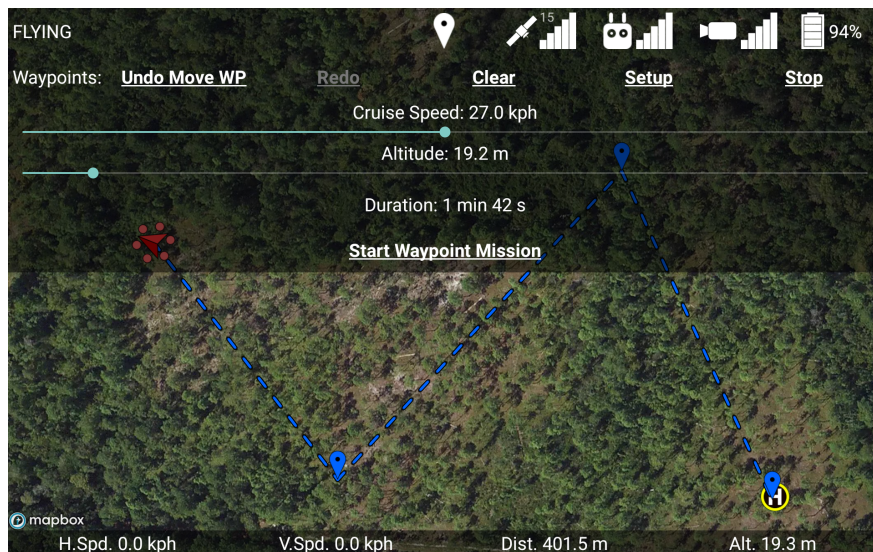
Figure 21: Adjusting the cruise speed and altitude of the waypoint mission.
