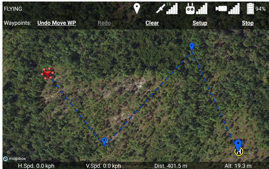
Figure 27: Touching somewhere on the map will move the selected waypoint to that location.
