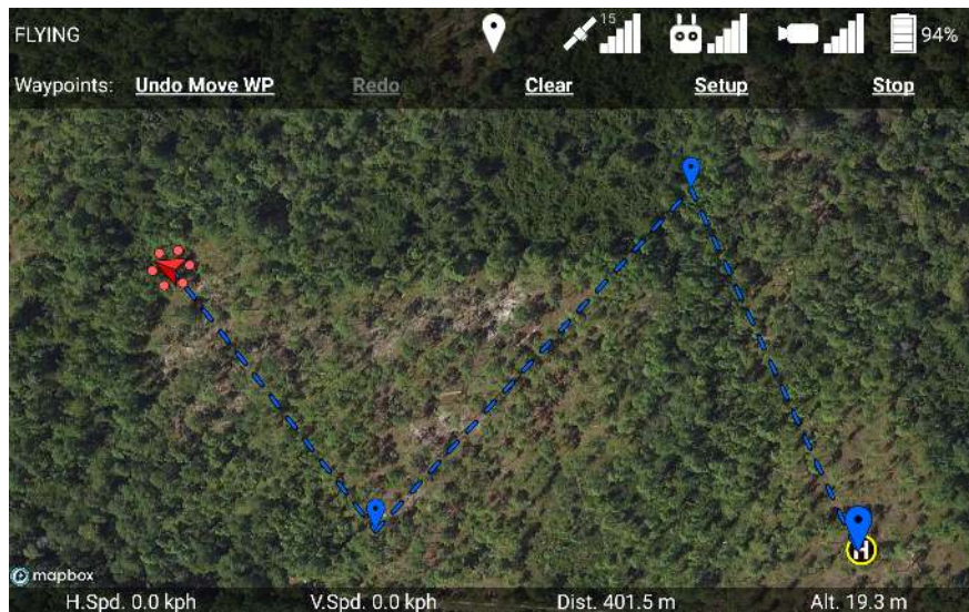
Figure 35: Touching somewhere on the map will move the selected waypoint to that location.
