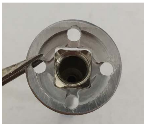
Figure 89: The needle can only fit through the rectangular hole in one orientation.
