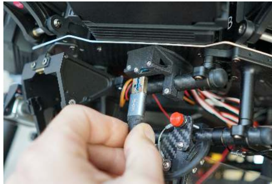
Figure 24: Attaching cable from the Hopper to the Drone.
