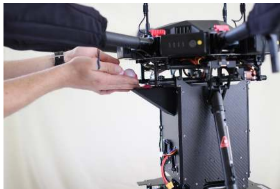
Figure 36: Filling the Hopper with ignition spheres.
