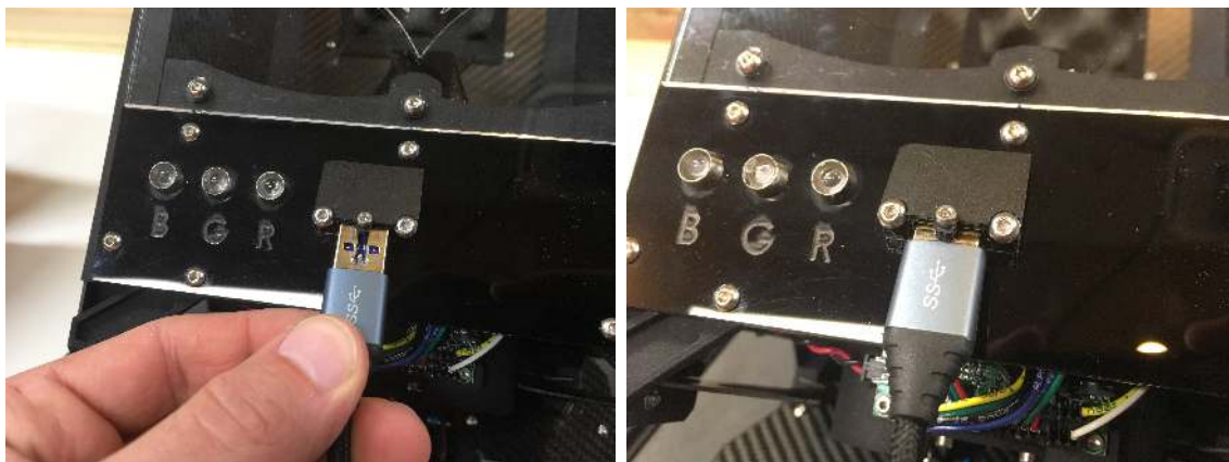
Figure 9: Left: Location to connect the wires from the Dropper to the Hopper. Right: Connected wires.
