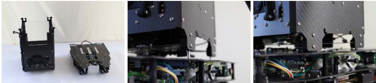
Figure 7: Attaching the Dropper to the Hopper.
