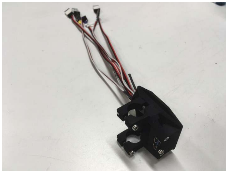
Figure 93: Interface cables for DJI.
