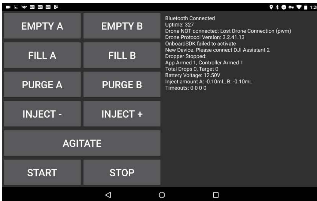
Figure 101: Error message displayed when the Matrice 600 has not performed the DJI Onboard SDK Activation with Ignis
