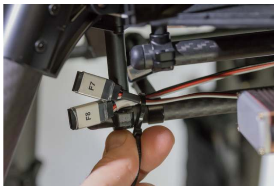
Figure 98: Ziptie the connectors in place.
