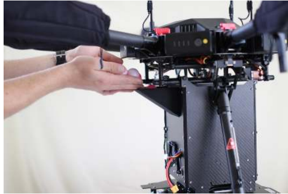
Figure 29: Filling the Hopper with ignition spheres.
