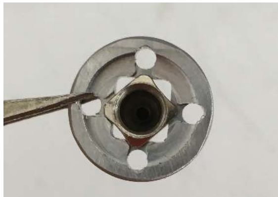
Figure 90: Needle tabs aligned with the cutouts on the retainer.
