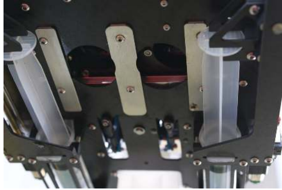
Figure 6: Hatches open and puncture area clear.
