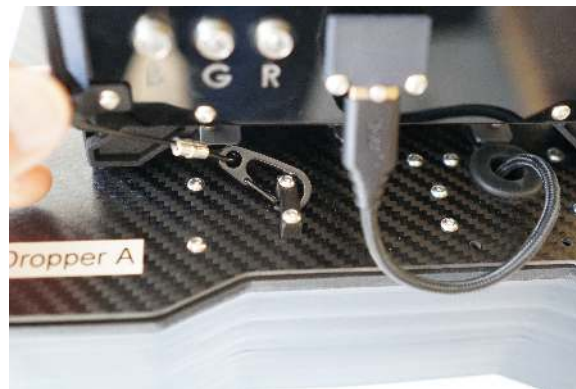
Figure 27: Attaching the front tether to the front connection point on the dropper. Clip the back tether to the back connection point.
