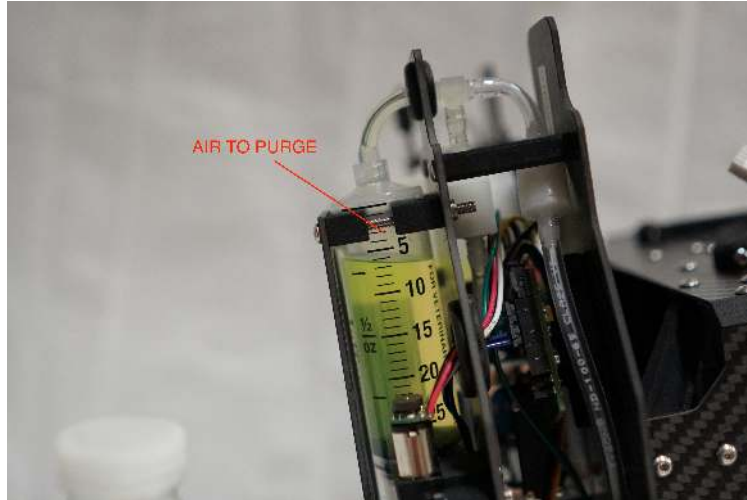
Figure 19: Ignis should be tilted so that the air in the syringes is near the tubes.
