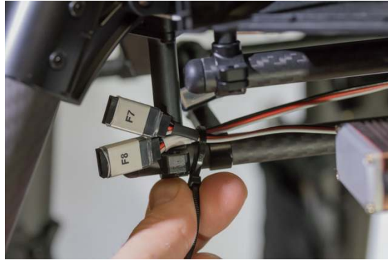
Figure 98: Ziptie the connectors in place.
