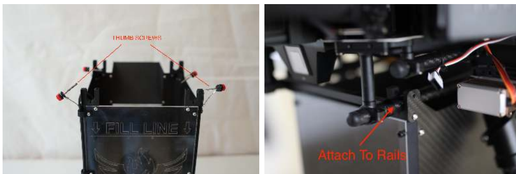
Figure 23: Attaching hopper to Drone. Left: Remove thumb screws. Right: Attach to drone.
