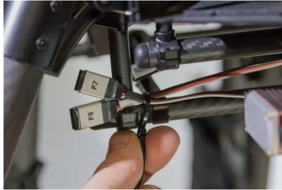
Figure 98: Ziptie the connectors in place.
