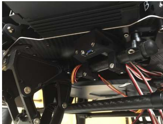
Figure 97: Attach USB port to upper rail under battery bay 6.
