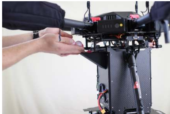
Figure 36: Filling the Hopper with ignition spheres.
