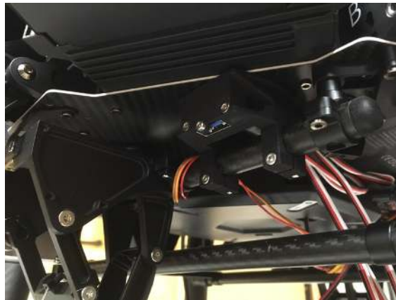
Figure 104: Attach USB port to upper rail under battery bay 6.
