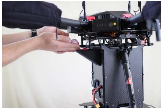
Figure 37: Filling the Hopper with ignition spheres.
