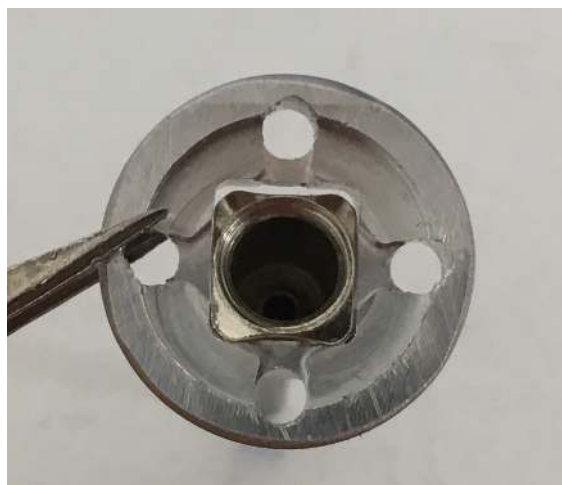
Figure 96: The needle can only fit through the rectangular hole in one orientation.
