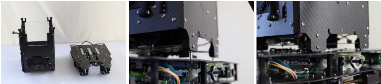
Figure 8: Attaching the Dropper to the Hopper.
