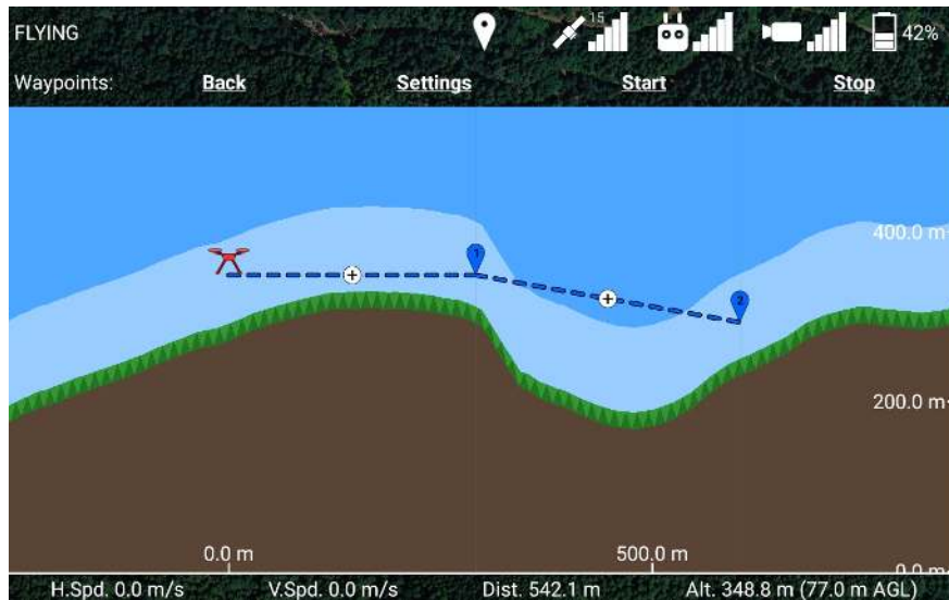
Figure 80: Drag waypoints in the side view to change their altitude.
