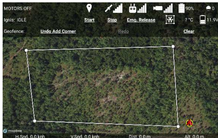
Figure 29: Creating a geofence for Ignis in the Ignis app.
