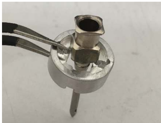
Figure 95: Slide the retainer over the new needle.
