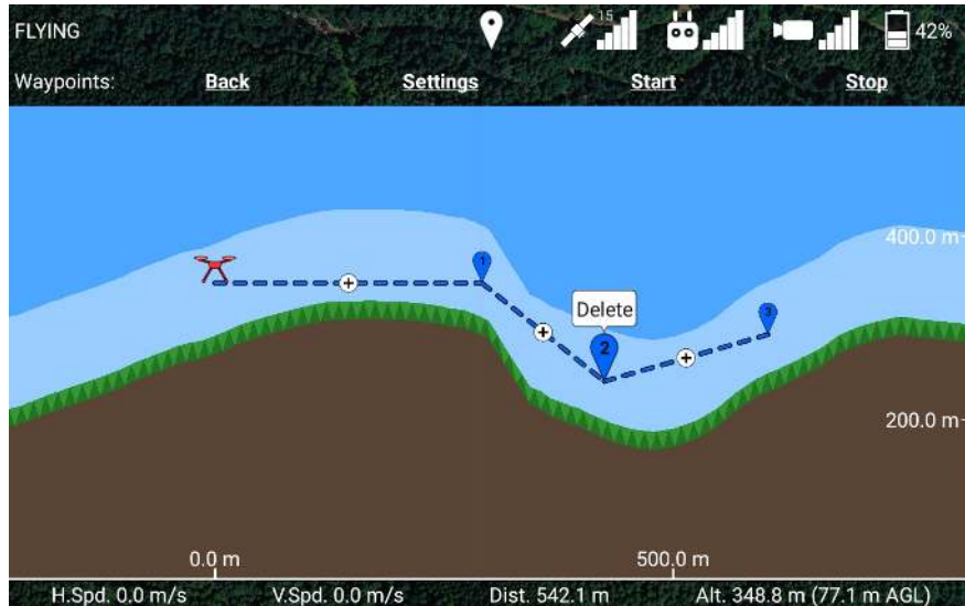
Figure 83: If you briefly touch a waypoint, it will give you the option to delete it. Touch the “Delete” bubble above the waypoint to confirm the deletion of it, or touch anywhere else to deselect it.
