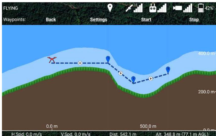
Figure 82: Waypoints that are colinear (or approximately colinear) with their neighboring waypoints can be dragged left and right as well as up and down.
