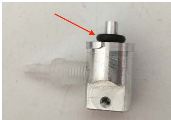
Figure 104: O-ring fully seated on needle mount.
