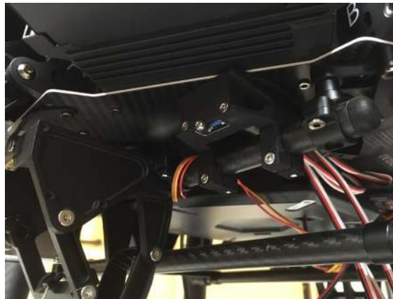
Figure 110: Attach USB port to upper rail under battery bay 6.
