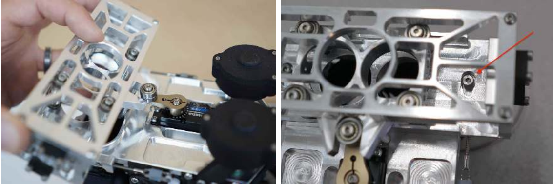
Figure 12: Attaching the Dropper to the Hopper.
