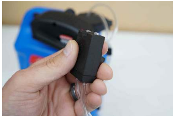
Figure 24: Proper grip on fill coupler
