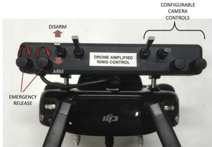
Figure 17: Ignis control switches.
