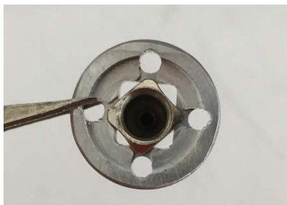
Figure 103: Needle tabs aligned with the cutouts on the retainer.
