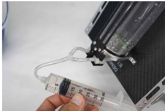
Figure 44: Connect the two tubes from the syringe to the check valves on the reservoir.
