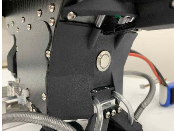
Figure 27: The status LED with multi-function button is located below the reservoir.
