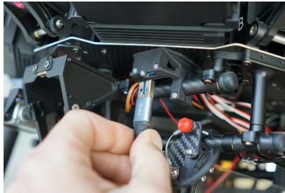
Figure 16: Attaching cable from the Hopper to the Drone.
