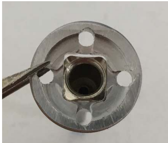
Figure 102: The needle can only fit through the rectangular hole in one orientation.
