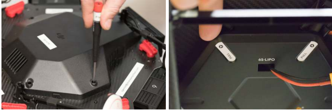
Figure 107: Unscrew top cover and remove bottom cover.
