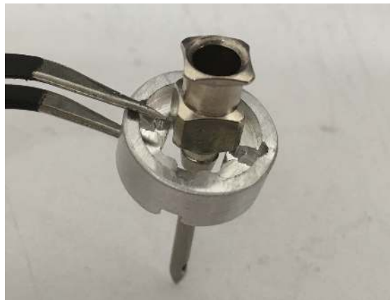
Figure 101: Slide the retainer over the new needle.
