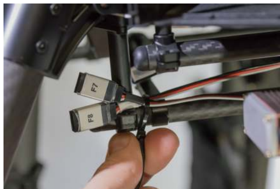
Figure 104: Ziptie the connectors in place.
