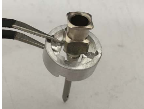
Figure 94: Slide the retainer over the new needle.
