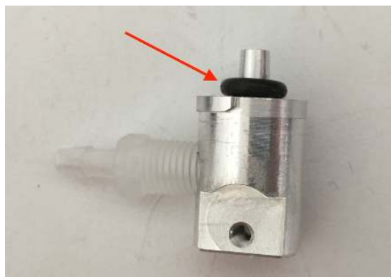
Figure 97: O-ring fully seated on needle mount.
