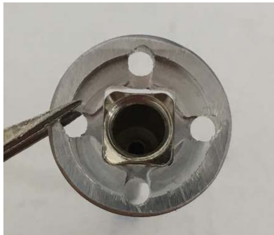
Figure 95: The needle can only fit through the rectangular hole in one orientation.
