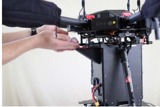
Figure 30: Filling the Hopper with ignition spheres.
