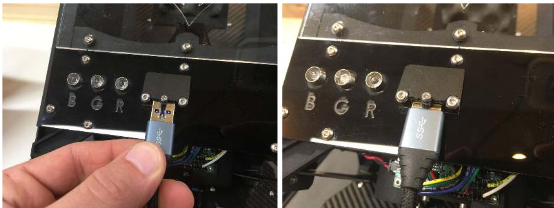
Figure 10: Left: Location to connect the wires from the Dropper to the Hopper. Right: Connected wires.
