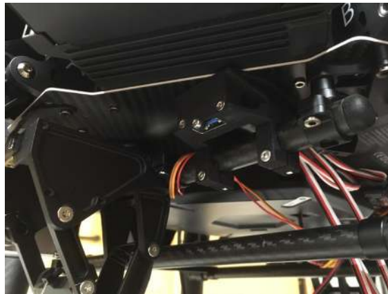
Figure 103: Attach USB port to upper rail under battery bay 6.
