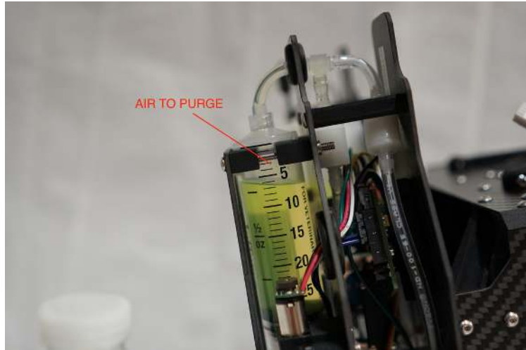
Figure 20: Ignis should be tilted so that the air in the syringes is near the tubes.
