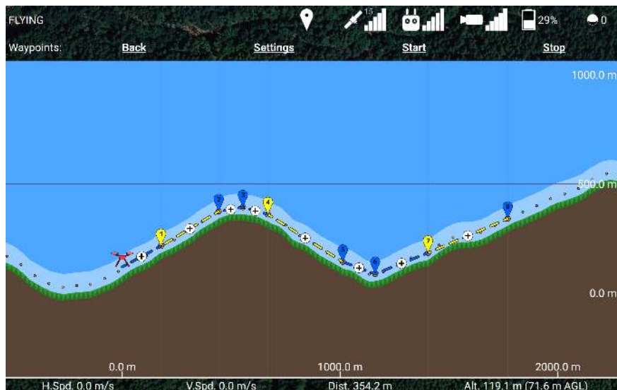
Figure 94: You can also toggle dropping along lines by touching them in the side view.
