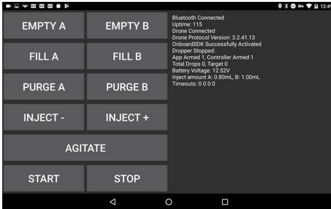
Figure 115: Message displayed when the DJI Onboard SDK is Successfully Activated
