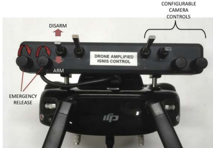
Figure 34: Ignis control switches.
