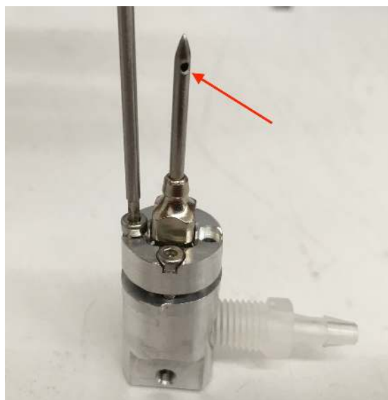
Figure 105: Needle hole oriented so that it will face downward when inserted in Ignis.
