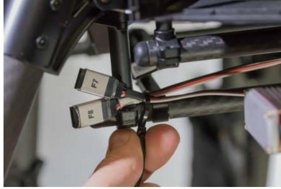
Figure 111: Ziptie the connectors in place.
