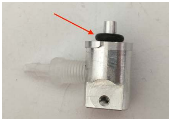
Figure 104: O-ring fully seated on needle mount.
