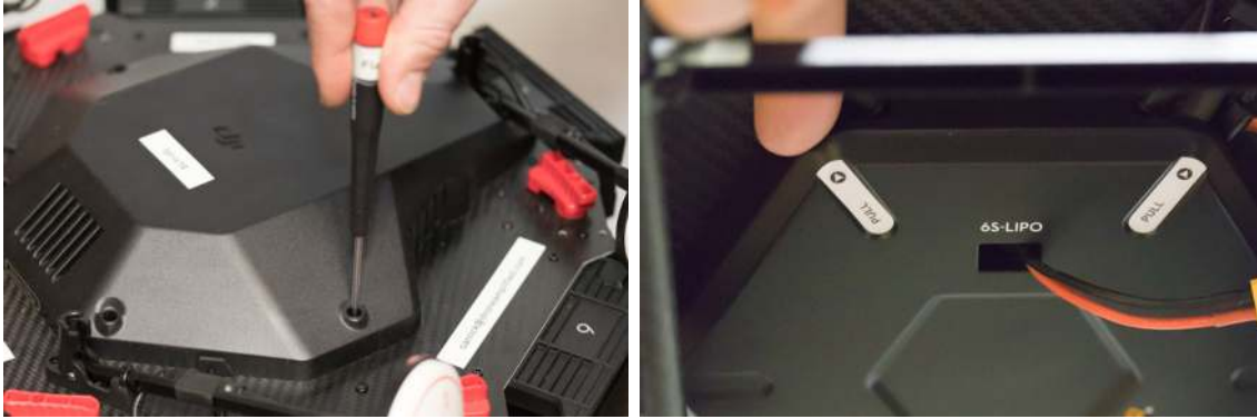
Figure 107: Unscrew top cover and remove bottom cover.
