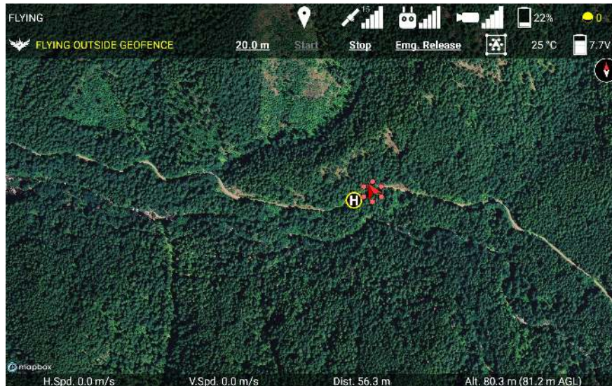
Figure 5: Ignis status display in app during flight, showing that Ignis is currently flying outside of a geofence.
