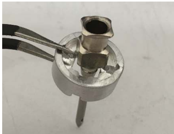
Figure 101: Slide the retainer over the new needle.
