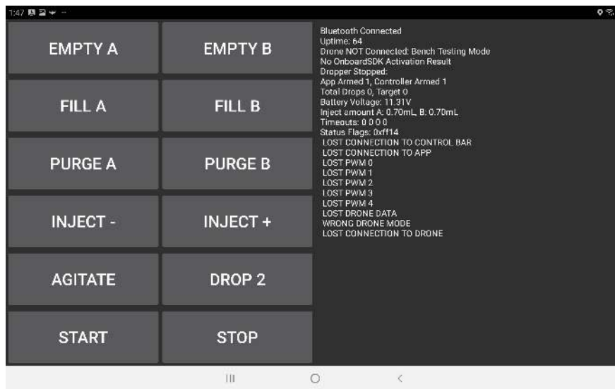
Figure 63: App when connected to Ignis 1 through Bluetooth.
