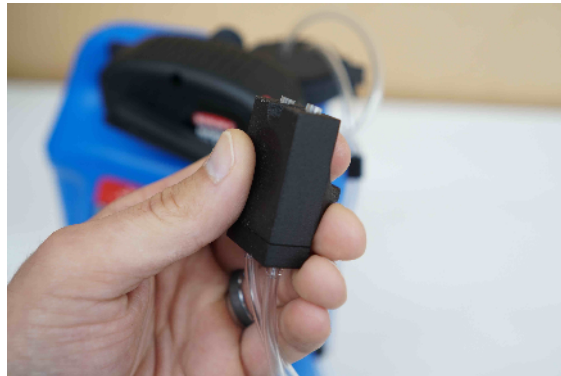
Figure 24: Proper grip on fill coupler
