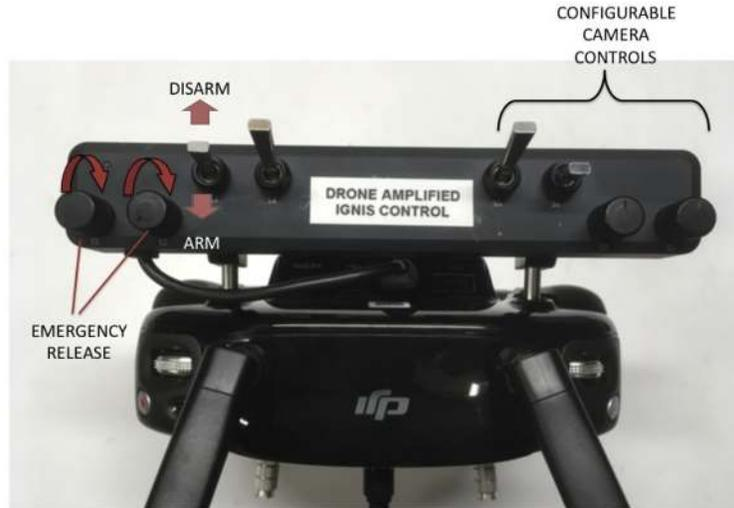
Figure 4: Ignis control switches.
