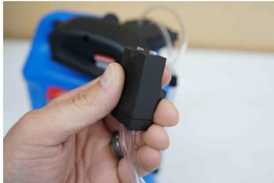
Figure 24: Proper grip on fill coupler
