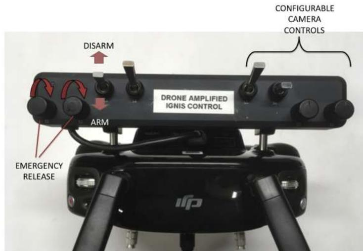
Figure 17: Ignis control switches.
