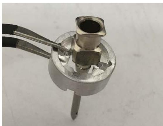
Figure 119: Slide the retainer over the new needle.
