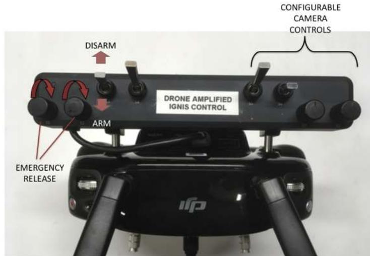
Figure 34: Ignis control switches.
