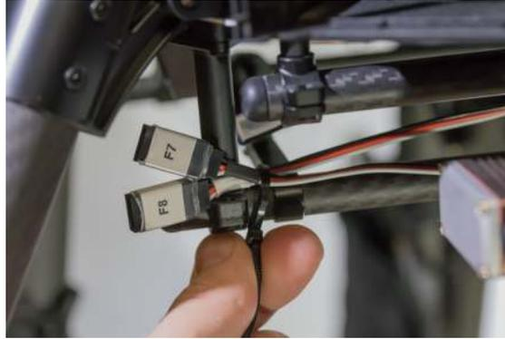
Figure 129: Ziptie the connectors in place.
