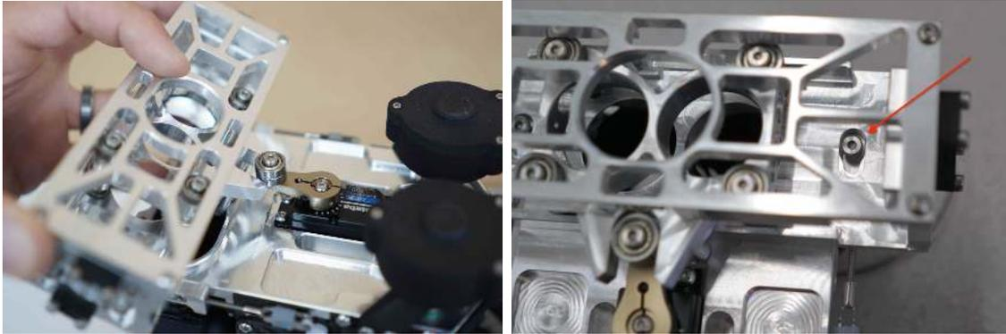
Figure 12: Attaching the Dropper to the Hopper.
