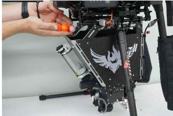
Figure 38: Filling the Hopper with ignition spheres.
