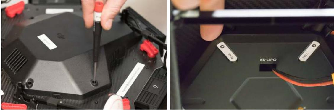
Figure 125: Unscrew top cover and remove bottom cover.
