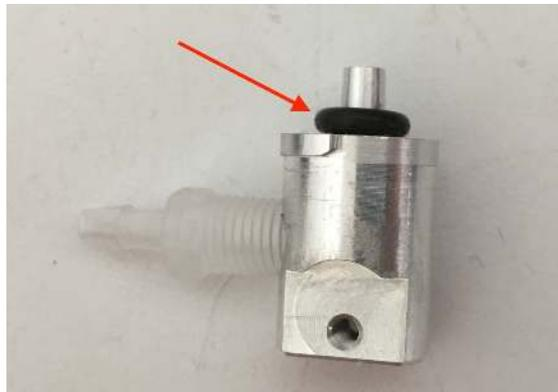
Figure 122: O-ring fully seated on needle mount.
