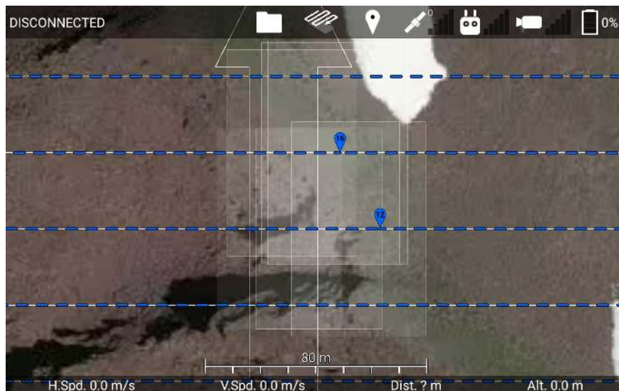
Figure 108: After adding intermediate waypoints from the side view, the photos have overlap the correct amount.
