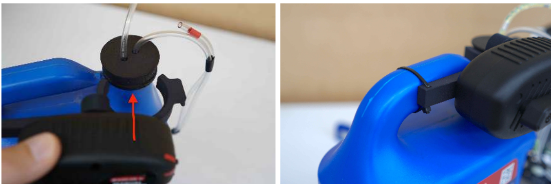
Figure 7: Snap pump mounting bracket around cap and zip-tie the other end to the handle.
