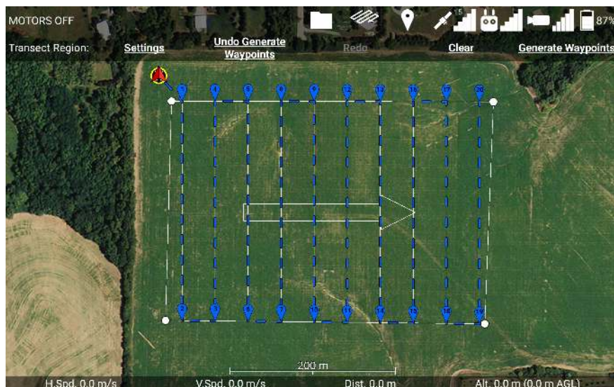
Figure 100: Touch the Generate Waypoints button to generate waypoints that follow the transects.
