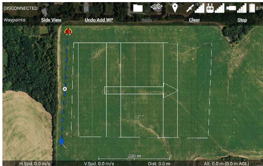
Figure 101: Place waypoints to define a custom ingress route to the transect region.
