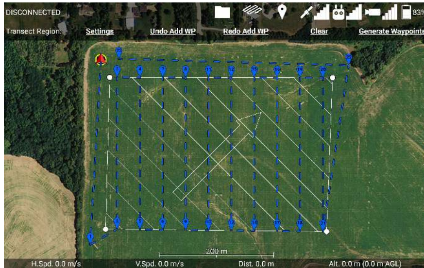
Figure 103: You can change the orientation and spacing of the transect lines even after generating waypoints.
