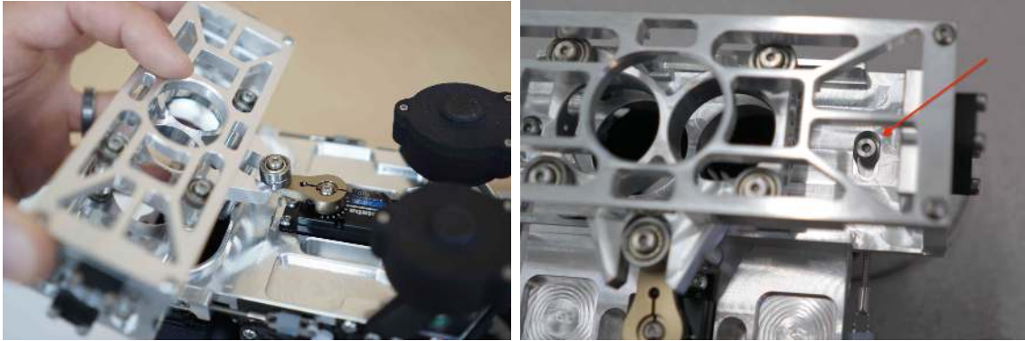
Figure 12: Attaching the Dropper to the Hopper.
