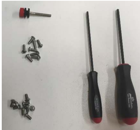
Figure 114: Replacement screws and drivers.
