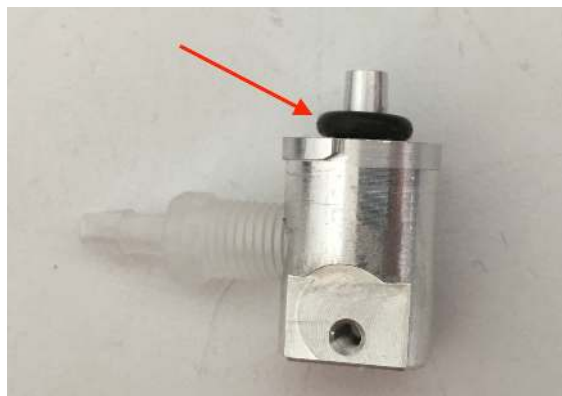
Figure 122: O-ring fully seated on needle mount.
