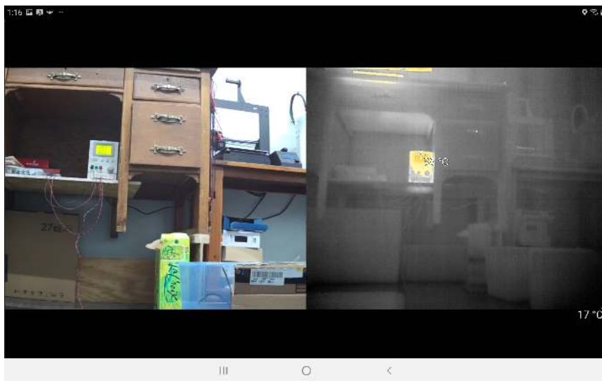
Figure 61: Maximized camera view. Area Metering is enabled, and the app shows crosshairs over the hottest and coldest parts of the video feed.
