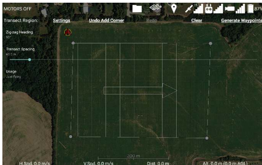
Figure 99: The Settings button shows controls for the length and orientation of the transect lines.
