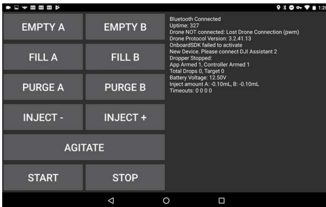
Figure 132: Error message displayed when the Matrice 600 has not performed the DJI Onboard SDK Activation with Ignis
