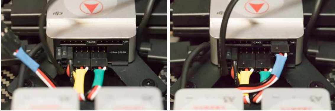
Figure 127: Three connectors installed.
