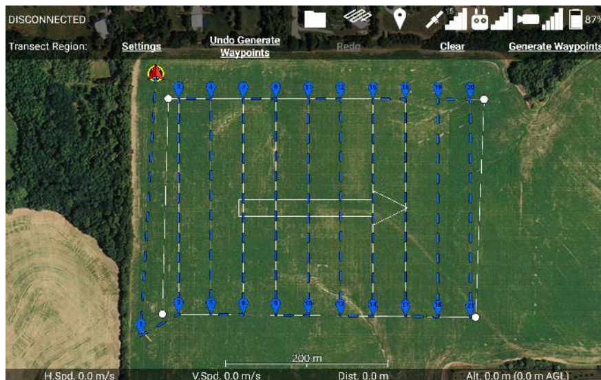
Figure 102: The generated waypoints of the transect region will start near the end of the ingress route.
