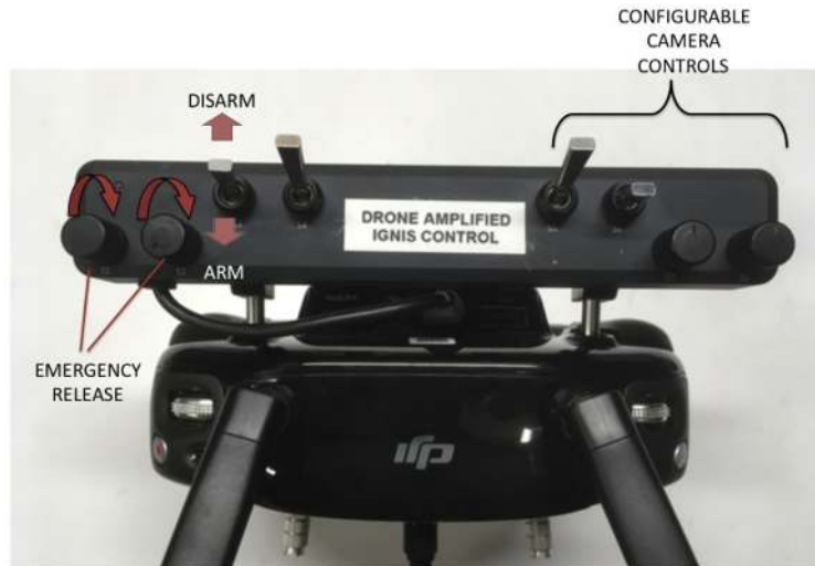
Figure 34: Ignis control switches.
