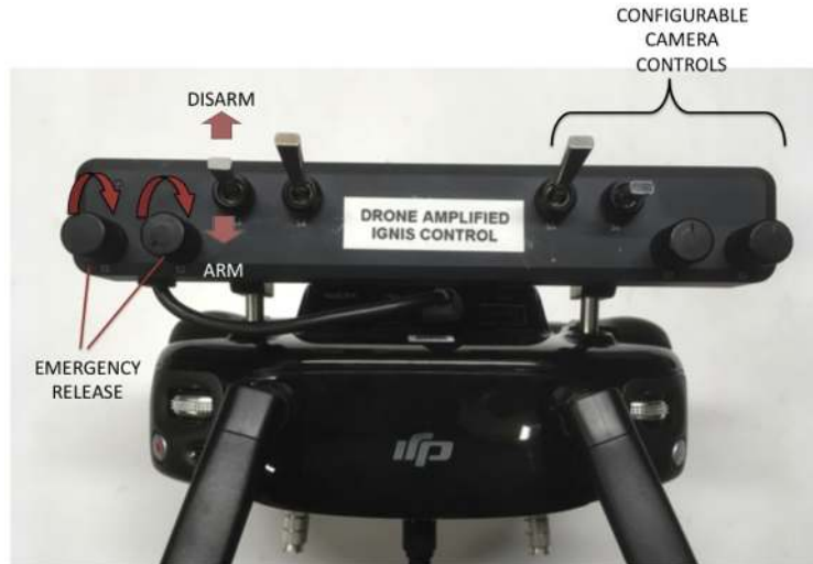
Figure 4: Ignis control switches.
