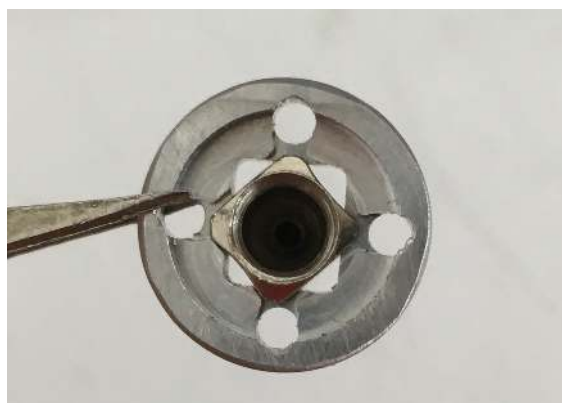
Figure 121: Needle tabs aligned with the cutouts on the retainer.
