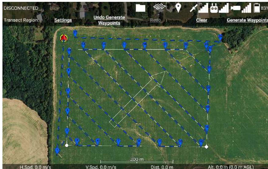
Figure 104: Newly generated waypoints will replace the part of your waypoint mission that passes through the transect region.
