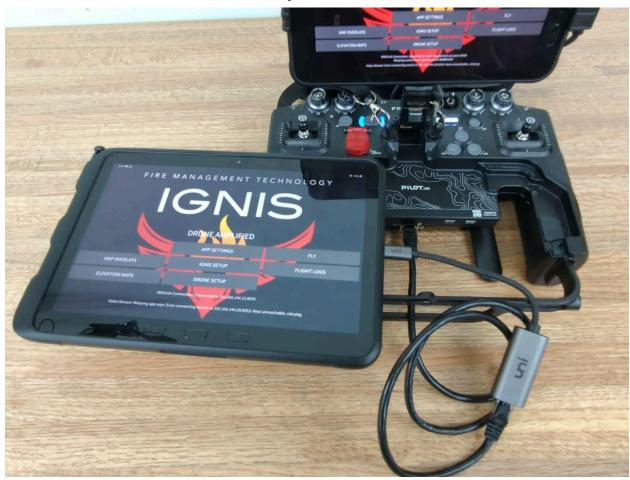
Open the Android Settings app on the big tablet, and go to Connections -> More Connection Settings -> Ethernet. Next, you must disable Ethernet by clicking on the slider in order to be able to configure it.
