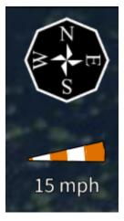
There is a new wind speed and direction indicator below the compass that displays a horizontal wind estimate calculated by the Astro's flight controller. It looks a bit like a wind sock. At 0 wind speed it is an orange circle, and as the speed increases it transforms into a longer triangle pointed in the direction the wind is blowing. Each stripe indicates 3 knots of wind.
