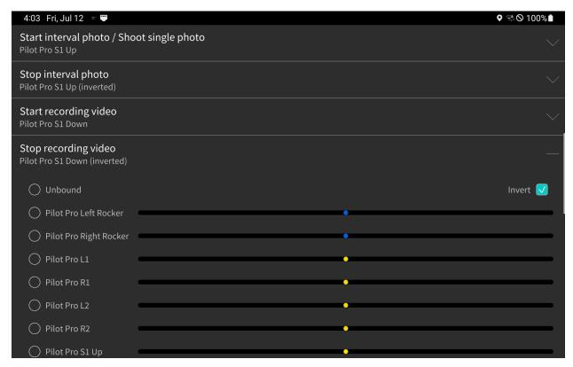
You can now bind functions to the S1 and S2 switches on the Pilot Pro, and it can be nice to have a switch control whether or not you're recording video, rather than a toggle button.
