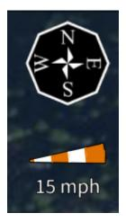
There is a new wind speed and direction indicator below the compass that displays a horizontal wind estimate calculated by the Astro's flight controller. It looks a bit like a wind sock. At 0 wind speed it is an orange circle, and as the speed increases it transforms into a longer triangle pointed in the direction the wind is blowing. Each stripe indicates 3 knots of wind.
