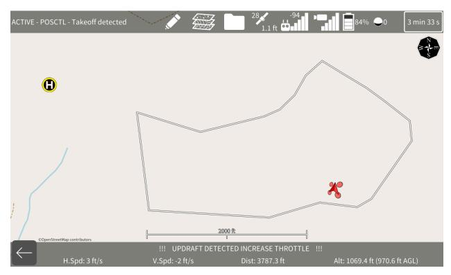
We've discovered a problem with the Alta X's firmware that has caused a few to crash. The logic that detects when the drone has landed and automatically shuts the motors off can trigger if you're hovering in an updraft, which will cause the drone to shut the motors off mid-air and crash. This can happen even with a fully loaded drone. Freefly is working on a fix for their Alta X firmware that will prevent this from happening.
