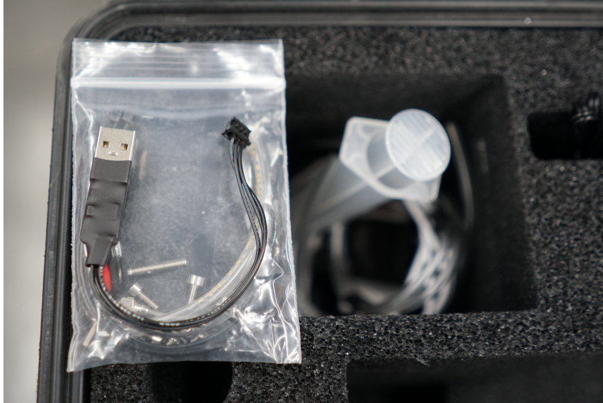
Figure 3: The Ignis updater USB cable, shown atop the spare parts bag it can be found in. The bag itself can be found in the upper left area of the Ignis case.
